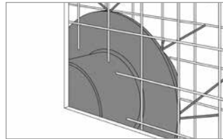
2 Example of fixing in steel formwork
